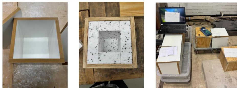
Figure 2: Insulated moulds with samples size 100mm 3 and insulation of 50mm
